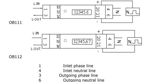
Connection of the wires should be done in accordance with the following connection diagram.
