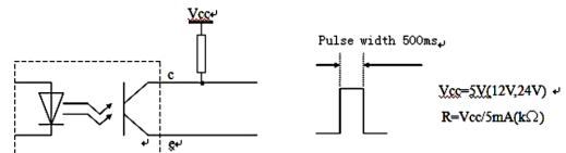
The terminals can be setup to switch to demand circle signal output and time output by RS485 and Infrared. When the meters power is off it will switch to 1Hz clock pulse output.
