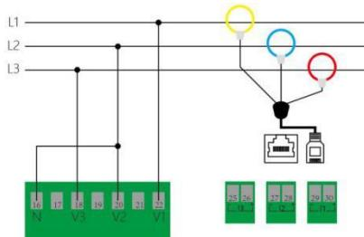
3PH3W(w/o PT) wiring diagram
