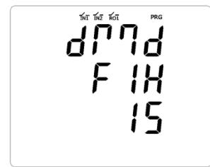
Press enter settings, the corresponding value will flash, Press or , modify values, Press toggles the value to be modified. After the data is modified, you will be prompted whether to save or not, Press or , to select yes or no, press perform the operation again.
