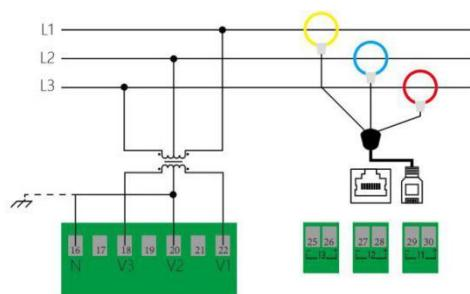
3PH3W(w/ PT) wiring diagram
