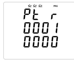
Press enter settings, the corresponding value will flash, Press or , modify values, Press toggles the value to be modified. After the data is modified, you will be prompted whether to save or not, Press or , To select Yes or no, press perform the operation again.
