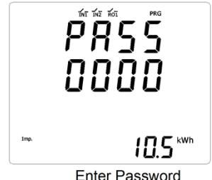
Before entering the configuration page, you need to enter the configuration password (default 1000). By pressing Enter password, By pressing or , Modify value size, By pressing Toggles the value to be modified (the corresponding value will flash), if the password is correct, it will enter the configuration interface.
