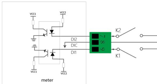
Digital input connection diagram
