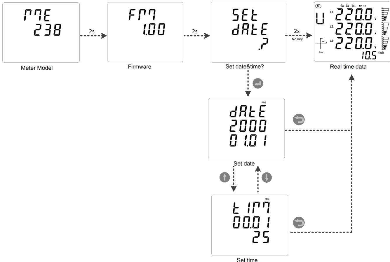
There is no backup battery for the meter clock. After power failure and restart of the meter, the time will return to 00:00:00:00 on January 1, 2020. Therefore, it is necessary to set the time of the meter when starting, otherwise the time of the meter will not be accurate.
