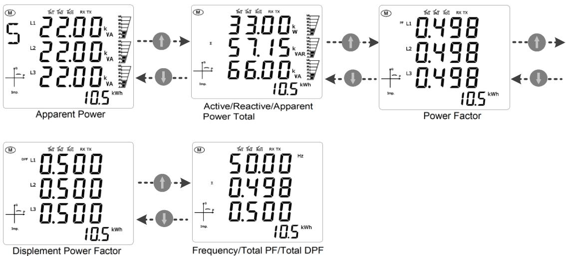
The following figure shows the real-time measurement data display interface of ammeter under three-phase three wire system.
