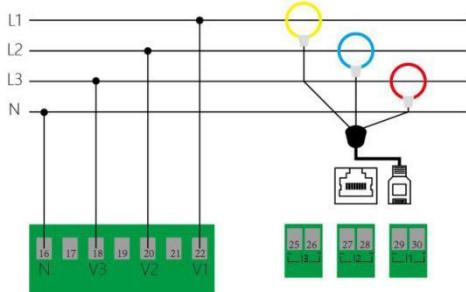
3PH4W(w/o PT) wiring diagram
