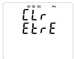
Press enter settings, the corresponding value will flash, Press or , modify values, Press toggles the value to be modified. You will be prompted whether to save or not, Press or , to select Yes or no, press perform the operation again.
