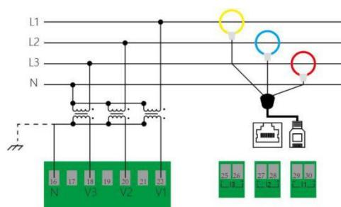
3PH4W(w/ PT) wiring diagram
